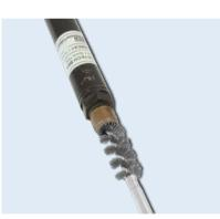
Cleaning of extended barrel spark plug
