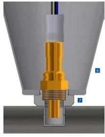
To increase life time of these critical sensors, there is also a stainless steel weld hub available that is welded into the exhaust pipe.
