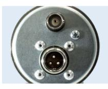
Additional BNC connector for high voltage measurement
