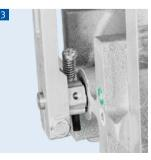
End stop with adjustment screw for idle speed
