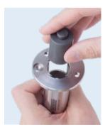
1 The tool is first fitted with the base insert that fits the corresponding spark plug.
