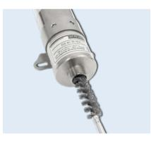
Cleaning of externally mounted ignition coil
