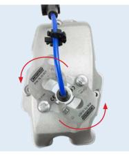
To unlock the spark plug lead the two screws just have to be loosened. The safety flanges can now be turned aside on the flange support.
